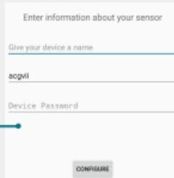
9 Enter your router's SSID and password. This information will be sent to your sensor so that it can connect to the cloud. NOTE: The sensor will not work as intended, if this information is entered incorrectly.
